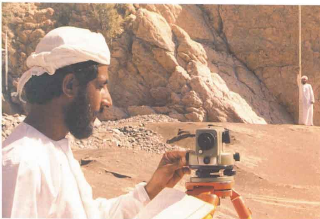
Surface water technicians take indirect measurements for the flood study programme (Photo: Min. of Water Resources)
