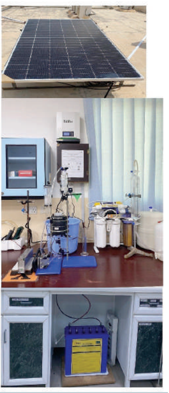
The project centres around a solar-powered purification system that meets Omani standards for safe drinking water.
