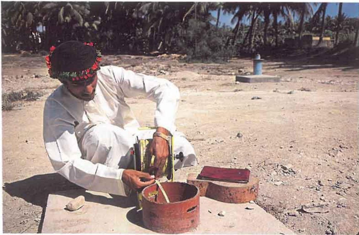
A technician measures ground water in Salalah
