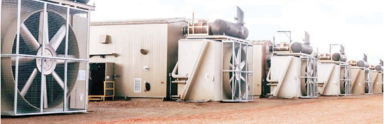
Methane-powered mobile data centres © Crusoe Energy
