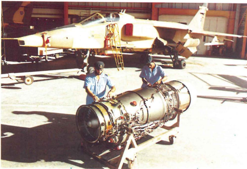
SOAF technicians carrying out maintenance on a Jaguar engine
