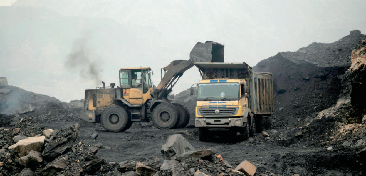
A worker operates a wheel loader to offload heaps of raw coal into a truck in Dhanbad, Jharkhand state. — AFP
