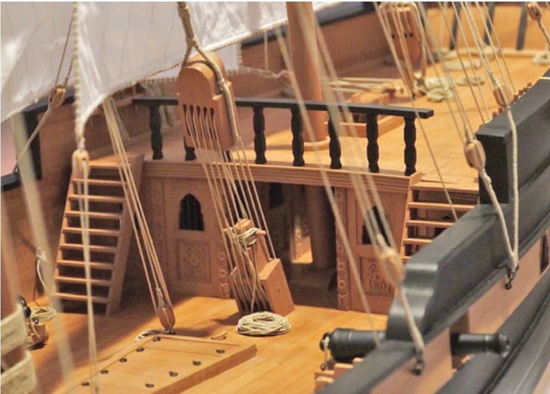
DEEP-SEA VESSEL: The baghla was the largest deep-sea trading and cargo vessel of the Arabian Gulf, and the most ornate of the big Arabian ships. She was fitted with two or occasionally three masts and was distinguished by ornamental projections that resembled the quarter galleries found on European line-of-battle ships of the 12th -13th century AH/18th -19th century CE.
