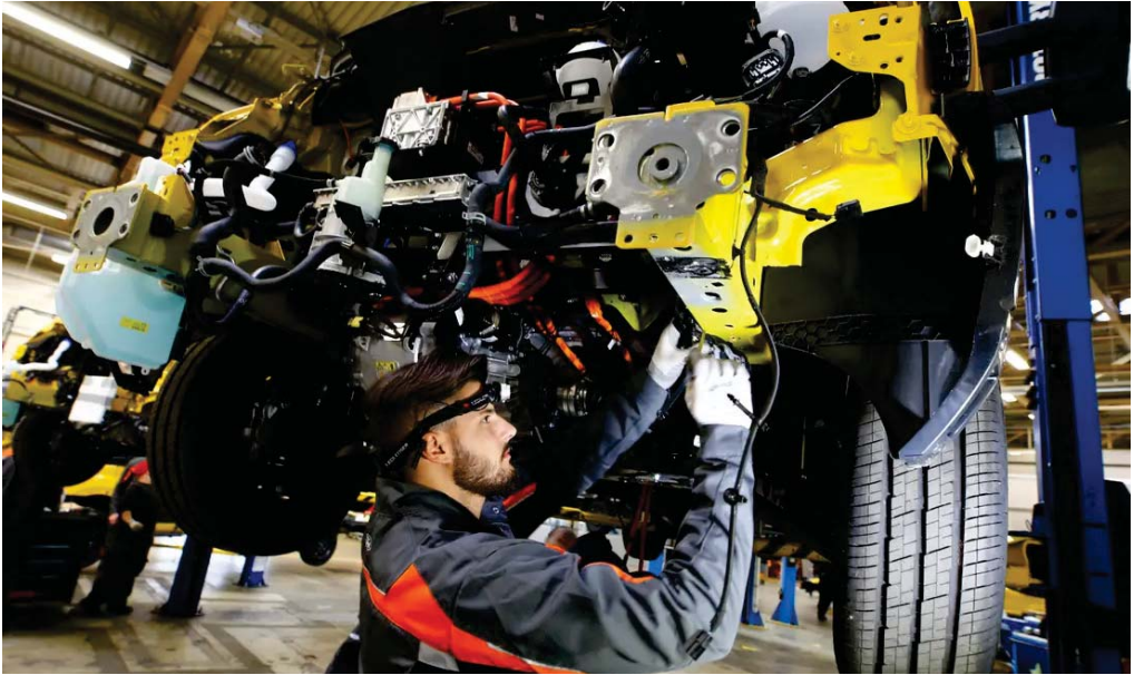
A worker of Ford Germany fixes the engine of a Streetscooter WORK XL electric van based on a Ford Transit at Ford's new manufacturing line in Cologne, Germany. — Reuters
