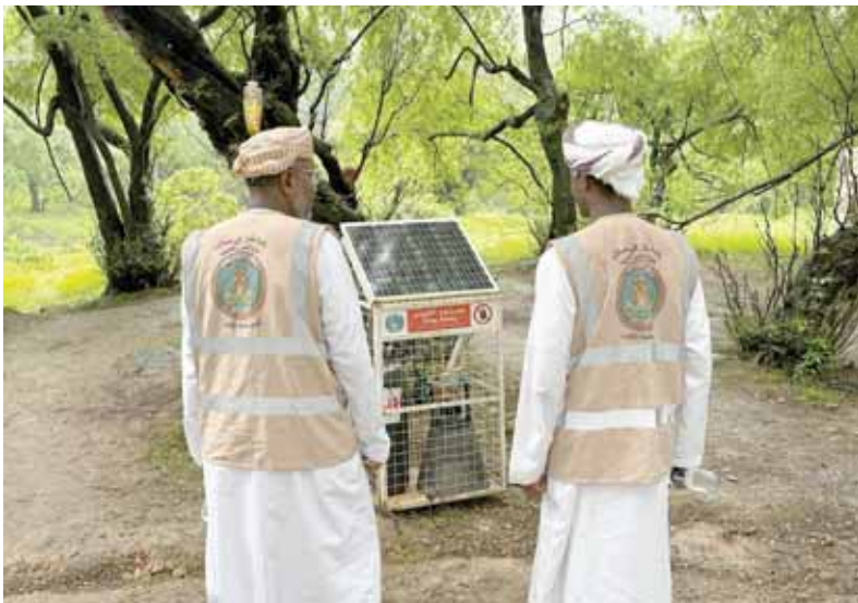
Carbon Trap installed in Salalah as a measure against the ‘aarnot’ seasonal fly
