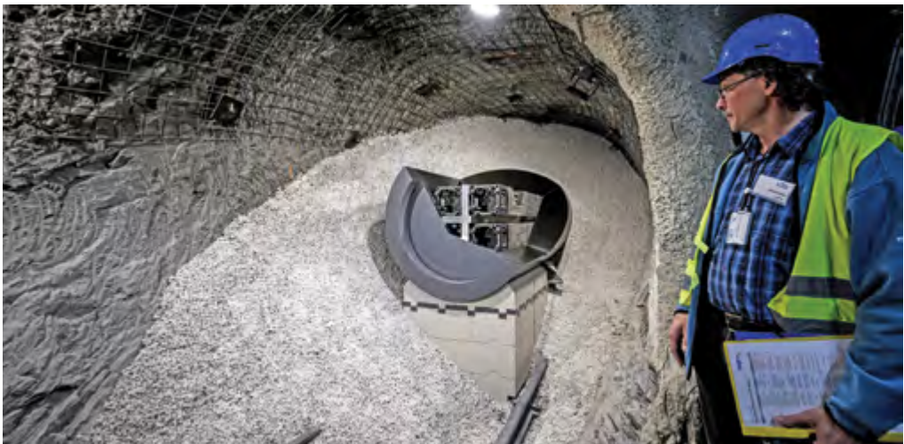
A real-size model showing an example of radioactive waste storage, in the Mont-Terri Rock Laboratory, dug out 300 metres below the surface, near Saint-Ursanne in the northwestern Swiss canton of Jura (AFP)
