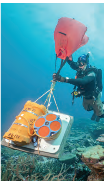
Curt Storlazzi, a coastal researcher with the US Geological Survey, installs a device to measure currents in the waters off Dhigulaabadhoo Island in the Maldives.
