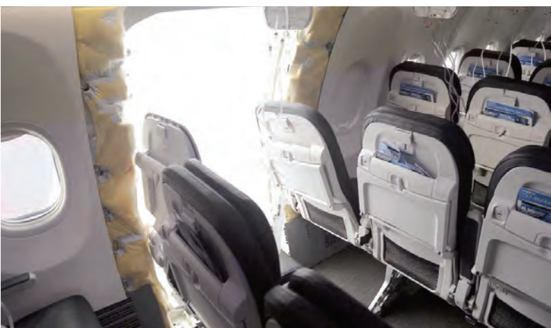
A gaping hole where the door panel had been on the Alaska Airlines Boeing 737 Max 9. — Reuters
