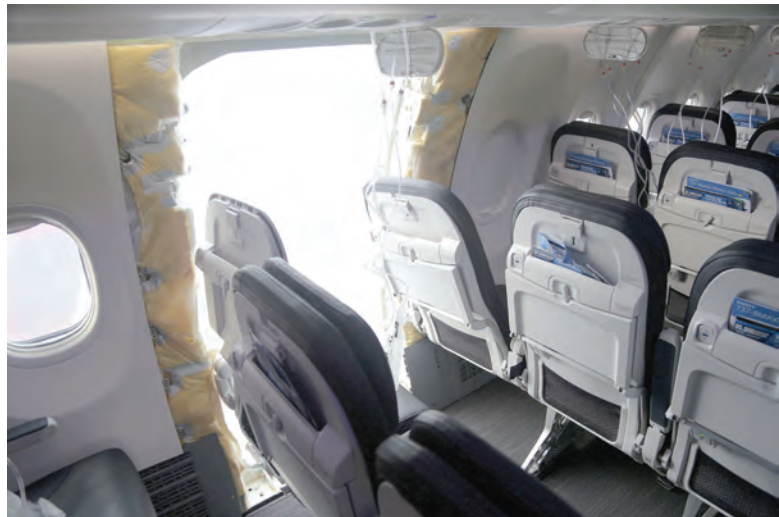
The fuselage plug area of Alaska Airlines Flight 1282 Boeing 737-9 MAX is seen during its investigation by the National Transportation Safety Board (NTSB) in Portland, Oregon. — Reuters file photo
