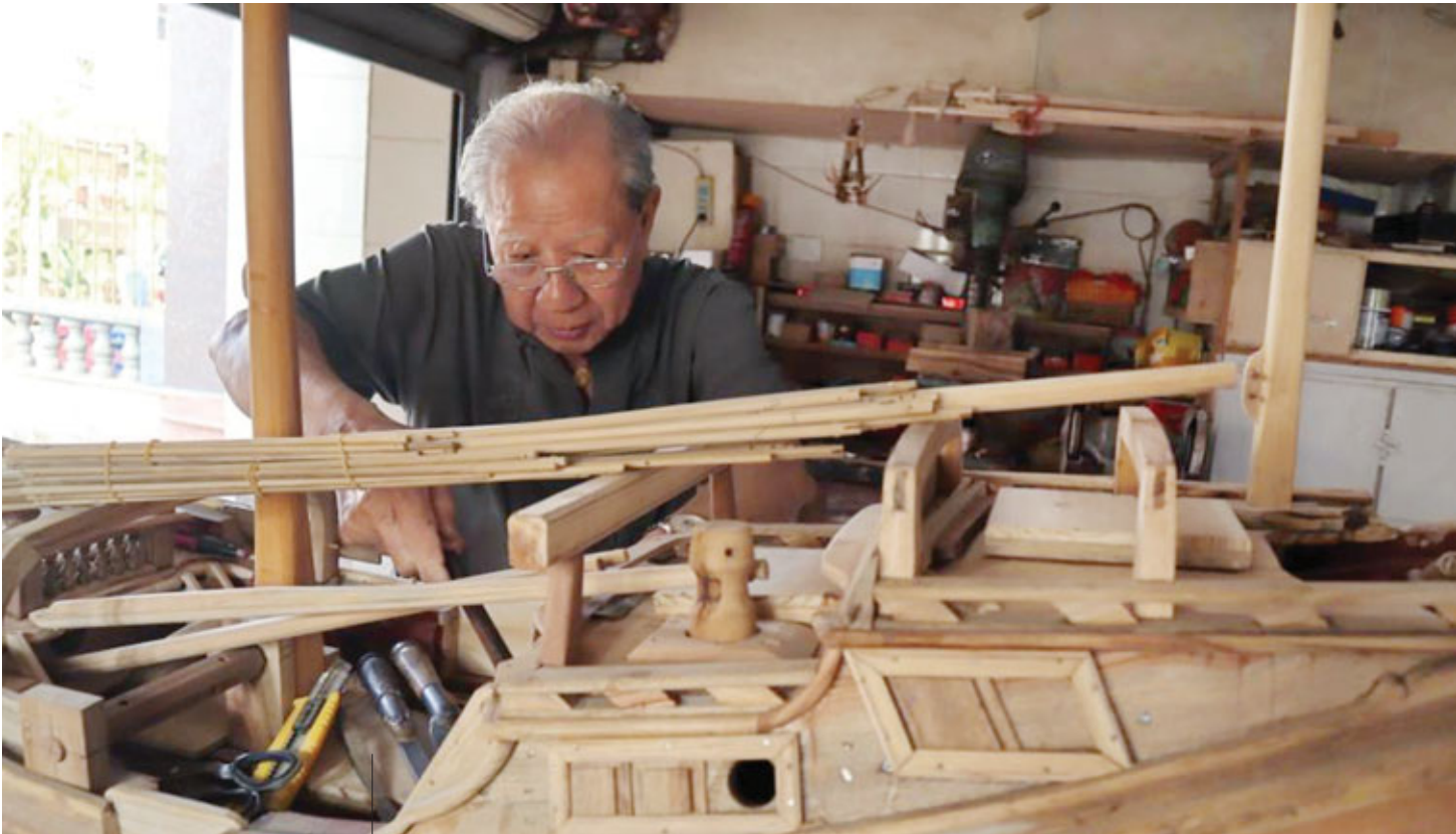
Craftsman's passion to pass on ancient shipbuilding technology Zhang Guohui, an inheritor of the watertight-bulkhead technology of Chinese junks, makes a model boat at a workshop in Chongwu Town,
