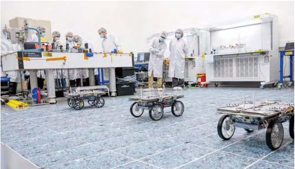
Engineers prepare three small Moon-bound rovers for a drive test in a clean room at the agency's Jet Propulsion Laboratory in Southern California in December 2023
