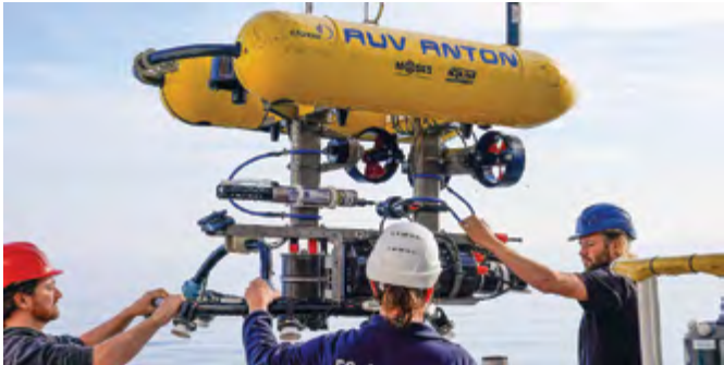
With autonomous underwater vehicles like these, GEOMAR can make photographic charts of the seabed
