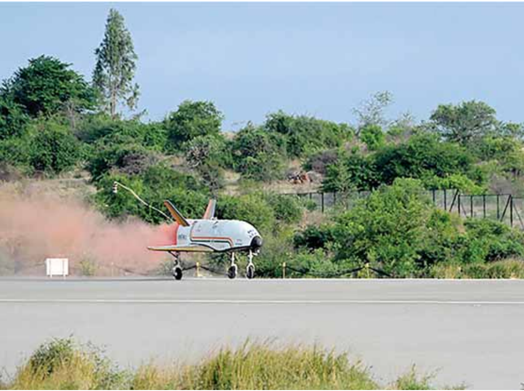
Following the success of the RLV LEX-01 and LEX-02 missions, RLV LEX-03 re-demonstrated the autonomous landing capability of the Reusable Launch Vehicle under more challenging release conditions
