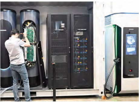
An engineer works on a flywheel energy storage system at Levistor's workshop in southwest London. — AFP
