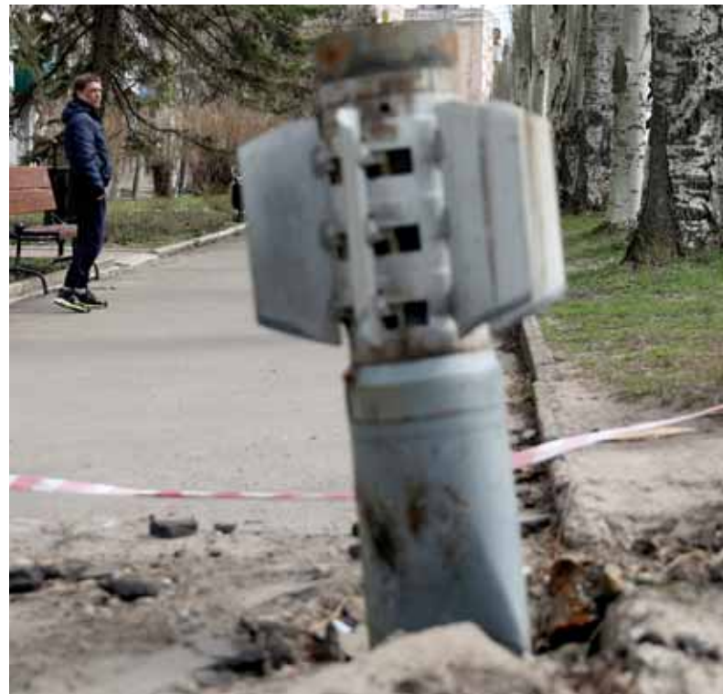
An unexploded tail section of a 300mm rocket which appear to contain cluster bombs launched from a BM-30 Smerch multiple rocket launcher embedded in the ground after shelling in Lugansk region. — AFP
