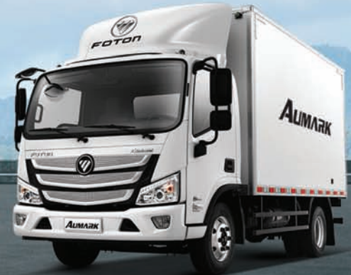
AUMARK S Light Duty Truck 3.8L Turbo Engine, 150hp
