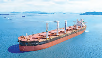
This 400,000-tonne vessel is equipped with five massive rotor sails.
