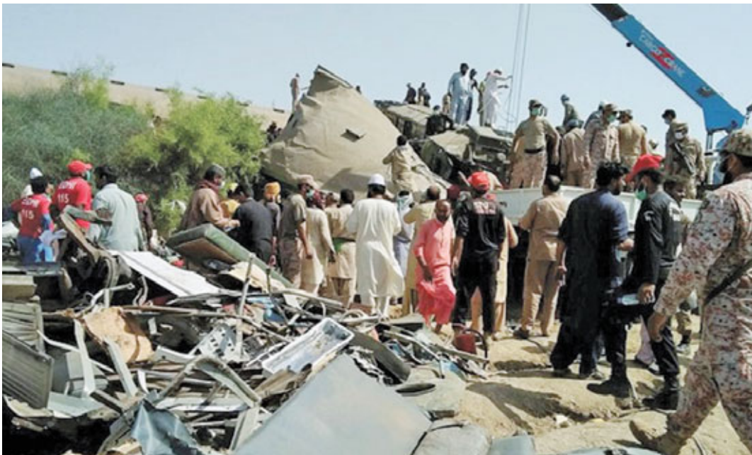
TRAIN COLLISION: According to the Pakistani newspaper, the train accident took place after a welding joint of the track broke.
