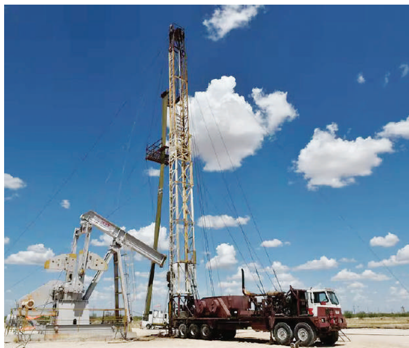
A work-over rig performs maintenance on an oil well in the Permian Basin oil production area near Wink, Texas US. — Reuters
