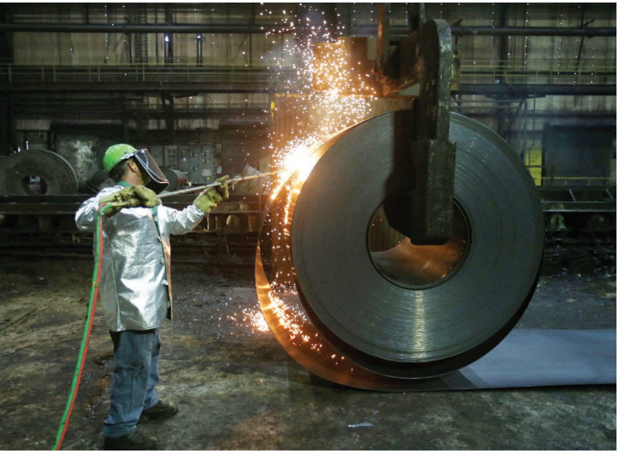
A worker cuts a piece from a steel coil at the Novolipetsk Steel PAO steel mill in Farrell, Pennsylvania. – Reuters
