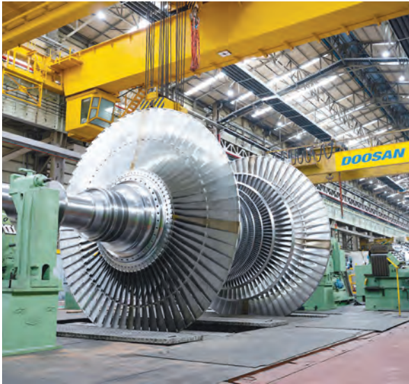
Steam turbine manufactured by Doosan Enerbility.
