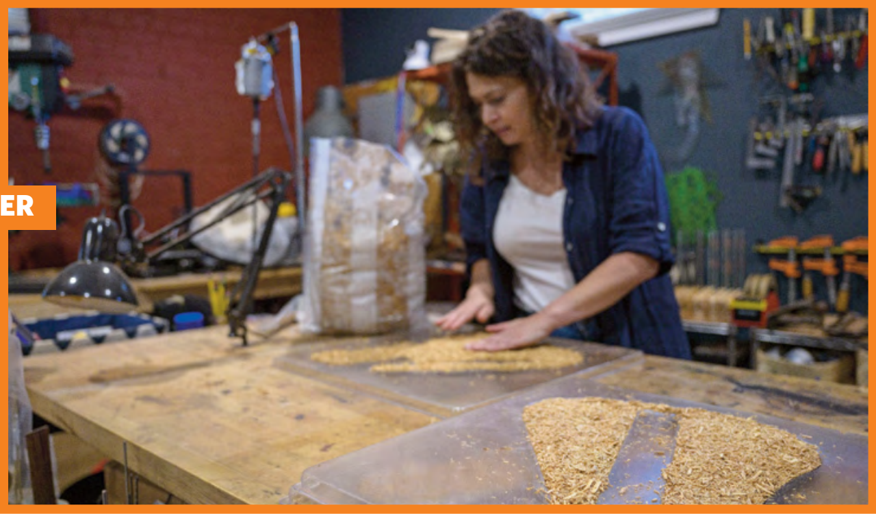
French luthier Rachel Rosenkrantz fills a mould with mycelium and cornhusks to make a guitar in her studio in Providence, Rhode Island
