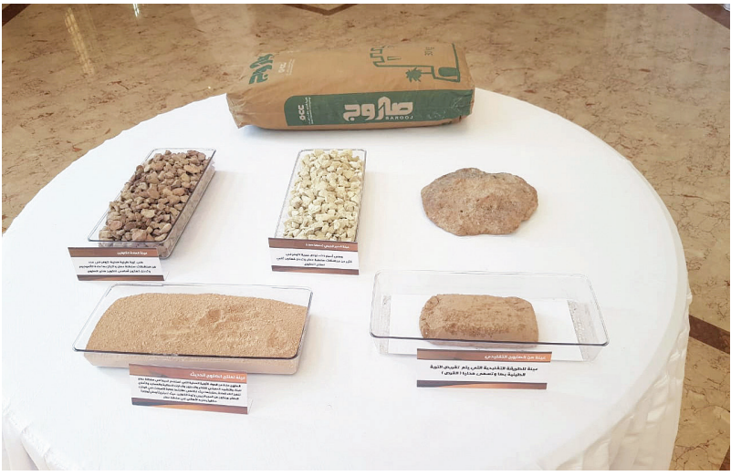
Historical Omani Sarooj samples exhibited high calcium oxide and low levels of reactive alumina-silicate, a composition that explains variable mechanical performance in traditional mixes.
