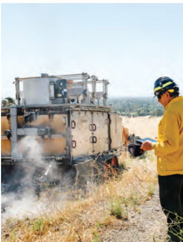
A Burnbot scorches the ground to create a firebreak to keep wildfires from growing, on grasslands at Stanford University in Palo Alto, California. — NYT
