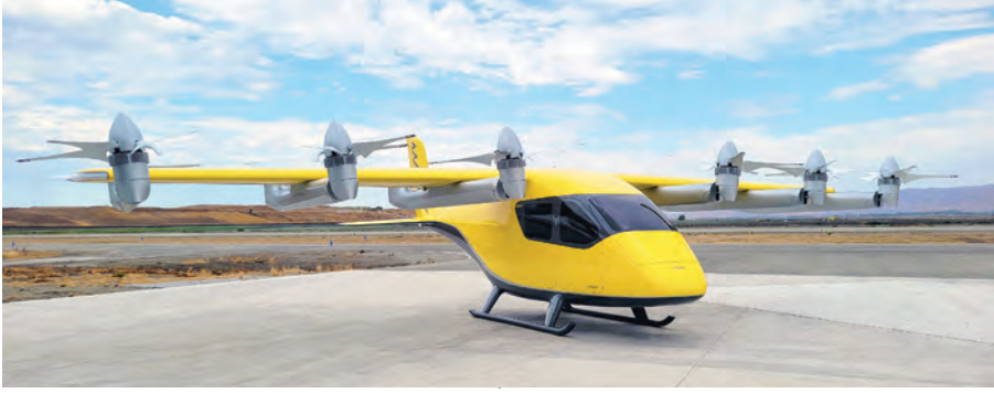
Wisk, is working to certify Gen6, an autonomous, all-electric, four-passenger eVTOL aircraft designed for self-flying air taxi services.
