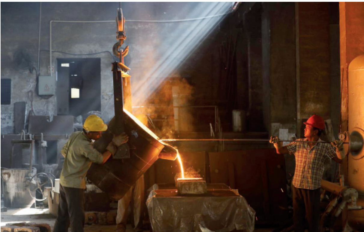
Workers pour molten iron into a mould at a workshop in Hangzhou, Jiangsu province, China. — Reuters
