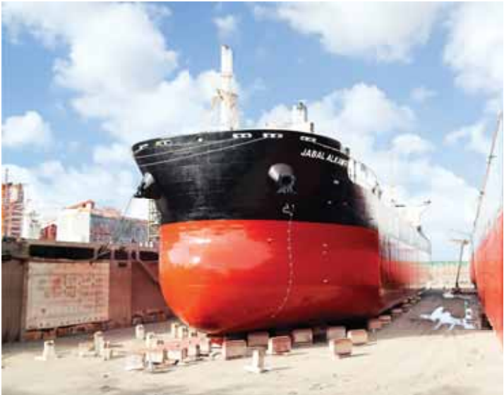
ECO-FRIENDLY: The smooth nano-epoxy silicone coating is resistant to fouling without the need to use biocides, thereby reducing impact on the marine environment. - ONA
