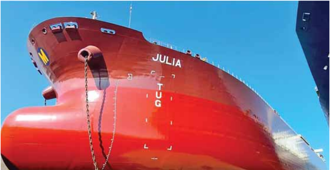
ECO-FRIENDLY: The smooth nano-epoxy silicone coating is resistant to fouling without the need to use biocides, thereby reducing impact on the marine environment. - ONA
