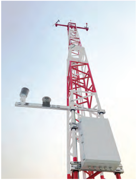
Met masts help with the generation of bankable data on the wind potential of locations targeted for Wind IPPs. Picture for illustration.
